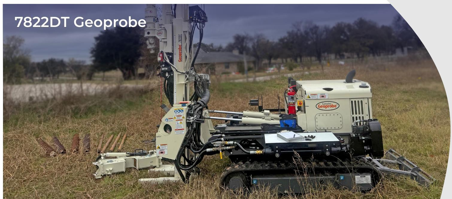
The Geoprobe 7822DT is a versatile and compact drilling rig, designed to adapt to different work settings. Its small footprint and wide track base allowing for maneuverability in confined spaces or remote sites.
